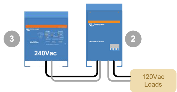
Autotransformer stepping down a single phase 240Vac supply into a single phase 120Vac supply
