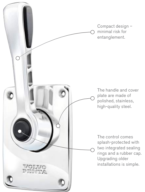
Mechanically operated, side-mounted controls for the D1/D2 series.
