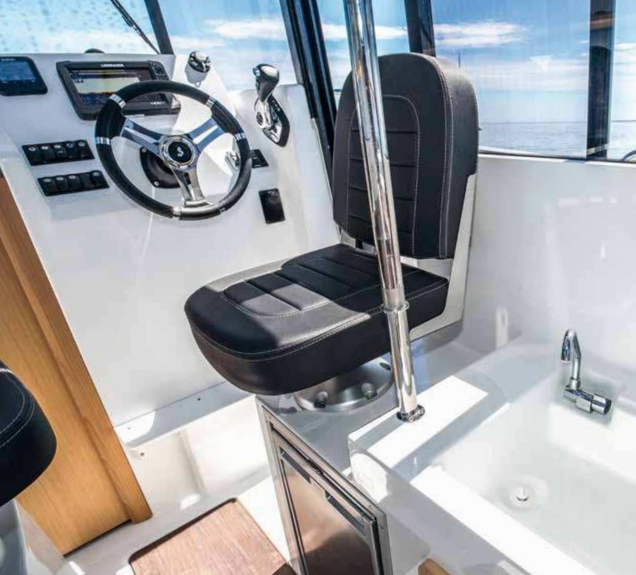
Inside the pilothouse is a very comfortable driving station and co-pilot's seat, from which there is a panoramic view. The two sliding side doors open directly onto the port and starboard walkways. The driver's seat cleverly rotates to free up space for the galley.
